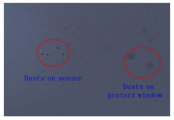
The big dim spot on the image (at right) are the shadows of dust on the protect window.
